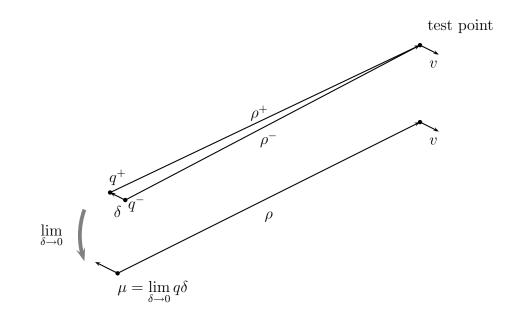
$$\varphi = \lim_{\delta \to 0} \left[ -\frac{q}{4\pi} \frac{1}{|\rho^+|} + \frac{q}{4\pi} \frac{1}{|\rho^-|} \right] = -\frac{1}{4\pi} \lim_{\delta \to 0} q \left| \delta \right| \left[ \frac{1}{|\rho^+|} - \frac{1}{|\rho^-|} \right] / \left| \delta \right| = -\frac{|\mu|}{4\pi} \frac{\partial}{\partial \hat{\mu}} \frac{1}{|\rho|}$$
