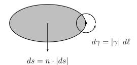
Velocity induced by a filament is a line integral  $v = \frac{1}{4\pi} \int_{\partial \mathscr{D}} d\gamma \times \nabla \frac{1}{|\rho|}$
