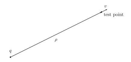
A source q induces velocity v at a test point with displacement vector  $\rho = (x, y, z)$ :
