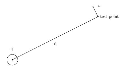
A vortex  $\gamma$  induces velocity v at a test point with displacement vector  $\rho = (x, y, z)$ :
